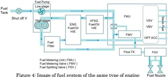
Figure 4: Image of fuel system of the same type of engine
