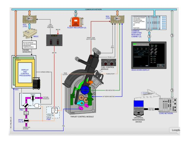
The two Fuel Switches are powered by separate Electrical buses and each switch has two separate signal paths. The possibility that all 4 signal paths failed simultaneously is negligible.
